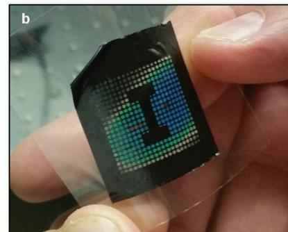
**Figure 5.** Images of the color response of stretchable materials for UV radiometry and the operation of a liquid crystal based colorimetric temperature sensor. a) Digital images of the UV colorimetric radiometer material captured just after UV-A exposure at intensities of 45, 36, 29, 23, 18, 9, 6, 0.6  $\text{W m}^{-2}$ . b) Image of a patterned pixel array of thermochromic liquid crystal formed by screen printing on a film of PET.
